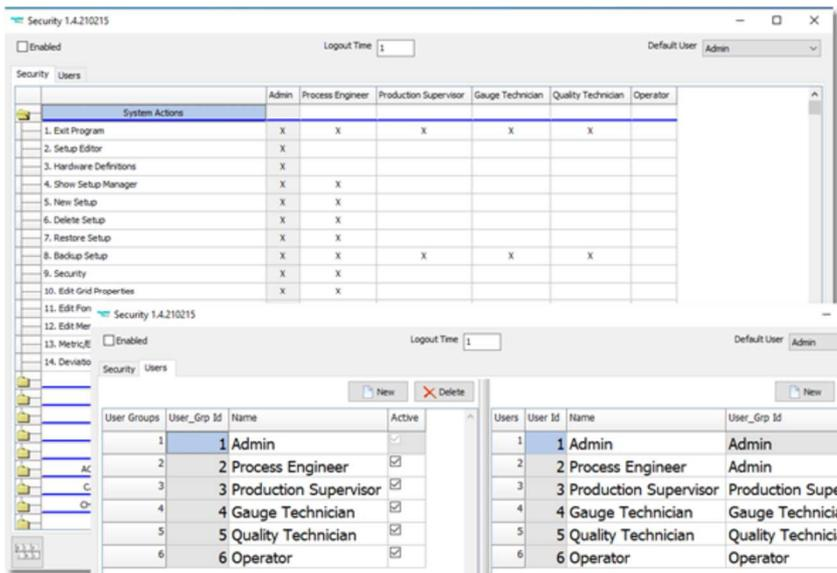
The screenshot displays the Security 1.4.210215 interface. It features a 'System Actions' table with columns for Admin, Process Engineer, Production Supervisor, Gauge Technician, Quality Technician, and Operator. Below this, there are two tables for user management: 'User Groups' and 'Users'.
